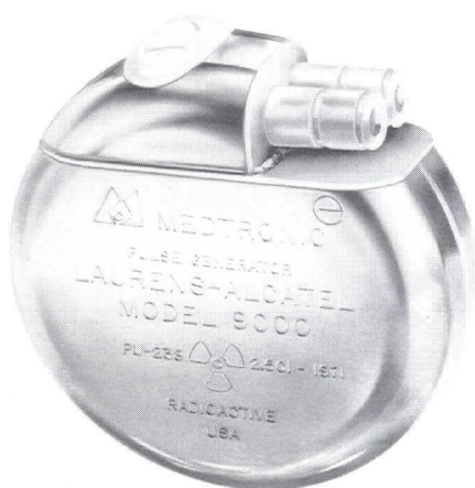
Figure 3 Photograph of Medtronic 9000 nuclear pulse generator.
